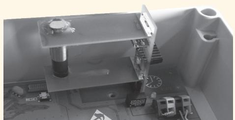
Antenna orientation in relation to the time-signal transmitter in Frankfurt
